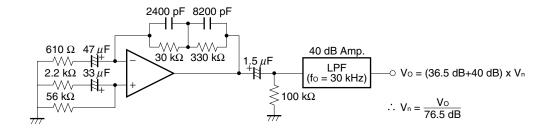
Fig.3 Flat Noise Measurement Circuit (FLAT+JIS A)
